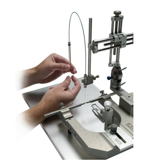
Quick and reliable connection of glass capillary needles and PEEK tubing to most Removable Needle (RN) and Knurled Hub (KH) terminations.
